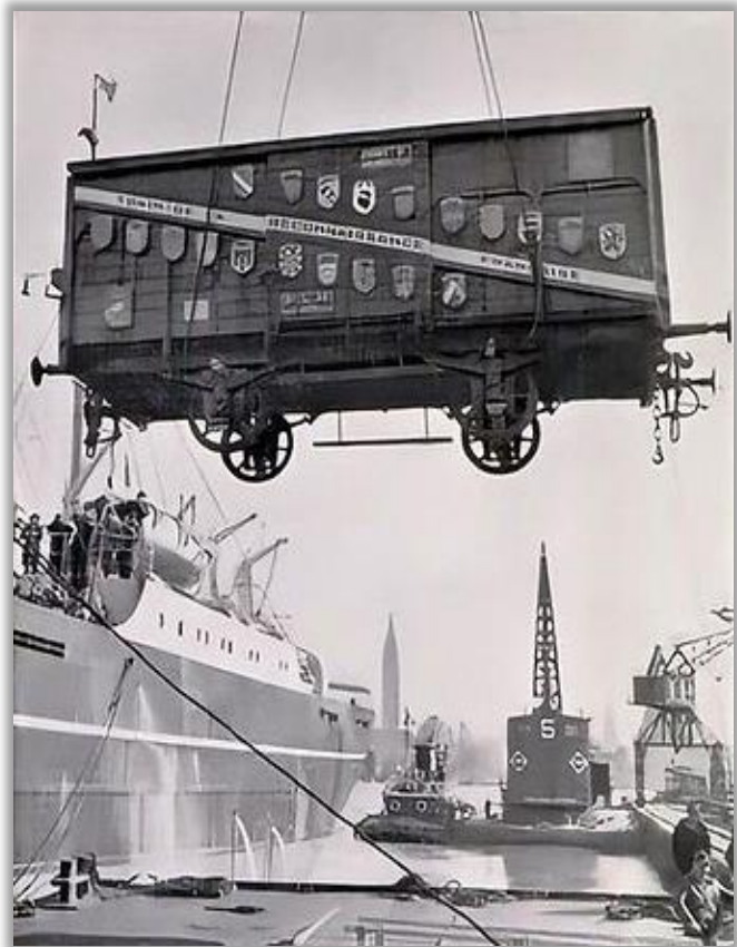
TRAIN DE LA RECONNAISSANCE FRANÇAISE One of the 49 Merci Train boxcars being unloaded from the New York harbor in 1949. The gauges were not compatible to fit cars on the U.S. train tracks so the boxcars were loaded onto flatcars.
