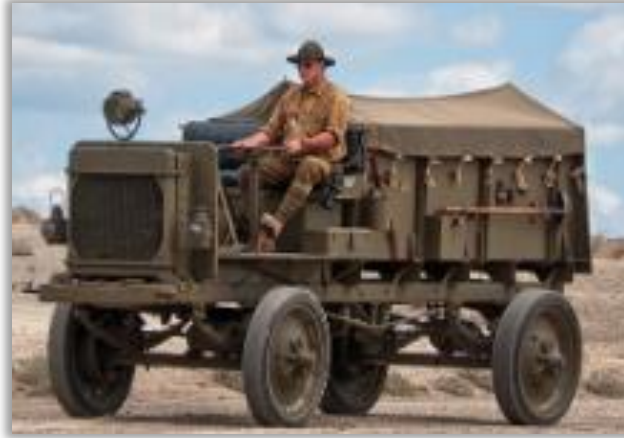
Four-Wheel Drive Nash Quad Truck Used by the Army in World War I
